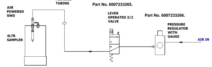
Our Air Powered SWD consists of a graduated plastic The operator just has to operate a button or lever to carry out the test which is much easier than manipulating a syringe when wearing thick gloves. It was also found that as the fuel level rises in the plastic tube, the fuel/air interface has no bubbles present so it is much easier to judge the true fuel volume than it is when using a conventional syringe, External SWD procedure.
